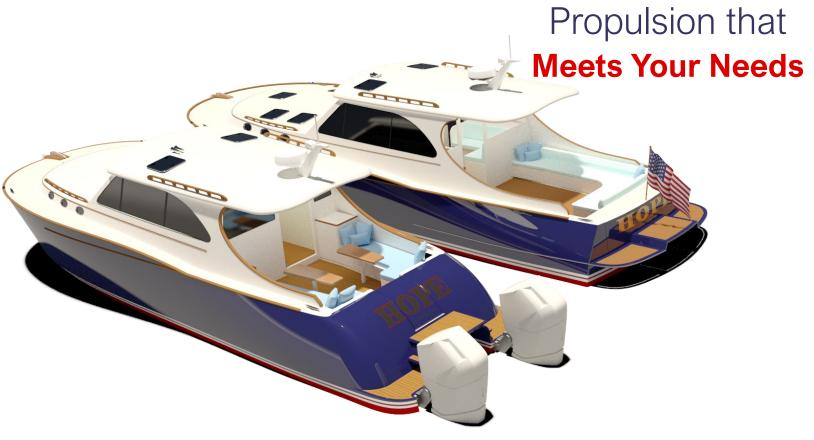
Different propulsion systems make sense for different applications. The Hope 40 is offered with either 2 x 600hp Mercury outboards, or 2 x 550hp Yanmar inboard diesel engines mated to Hamilton Jet Drives. The outboards represent a high value package with amazing performance. The inboard / jet drive combination offers reliability and safety.
