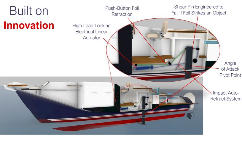
The Hope 40 utilizes a revolutionary hydrofoil system derived from the latest America's Cup technology. Existing power-catamaran foiling systems have two major flaws. First, the foil is always deployed between the hulls. Ready to grab a lobster pots, or other UFOs (unidentified floating objects). Second, foil impacts with floating objects at speeds result in dangerous decelerations, and the possibility of compromised hull/foil supports.
