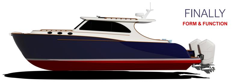
The Hope 40 combines traditional New England styling with a state of the art power catamaran utilizing hydrofoil technology. Classic "Down East" lines do not reveal that the Hope 40 utilizes a revolutionary foil package. The main foil of the Hope 40 has an adjustable angle of attack, and is fully retractable. In harbors where a foil between the hulls is a liability, the push of a button allows the foil hinge clear of entanglement.
